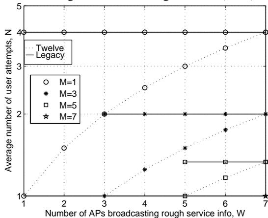
Fig. 3 –  $N_{Legacy}$  and  $N_{Beacon}$  versus  $W$ , with  $M$  as a parameter and  $K=7$ .
