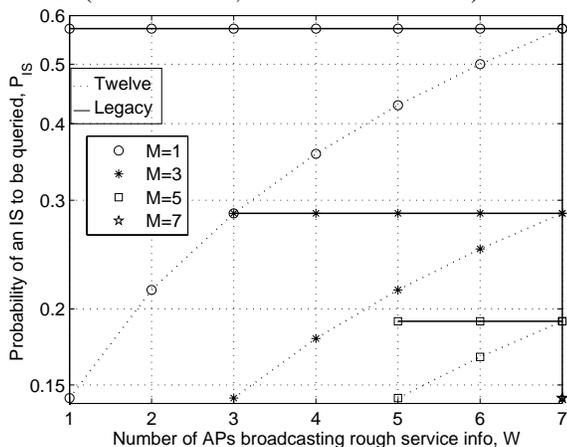
Fig. 4 –  $P_{IS,Legacy}$  and  $P_{IS,Beacon}$  versus  $W$ , with  $M$  as a parameter and  $K=7$ .
