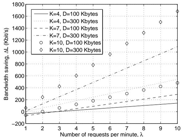
Fig. 5 –  $\Delta L$  versus  $\lambda$ , with  $K$  and  $D$  as parameters and  $W=M=1$ .
