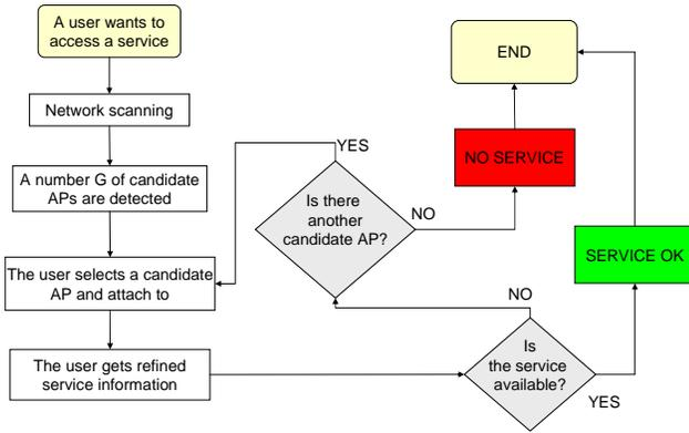
Fig. 2 – Service discovery process: flow diagram.
