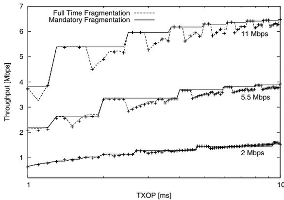
**Figure 7. Impact of different data rates on TXOP utilization**
